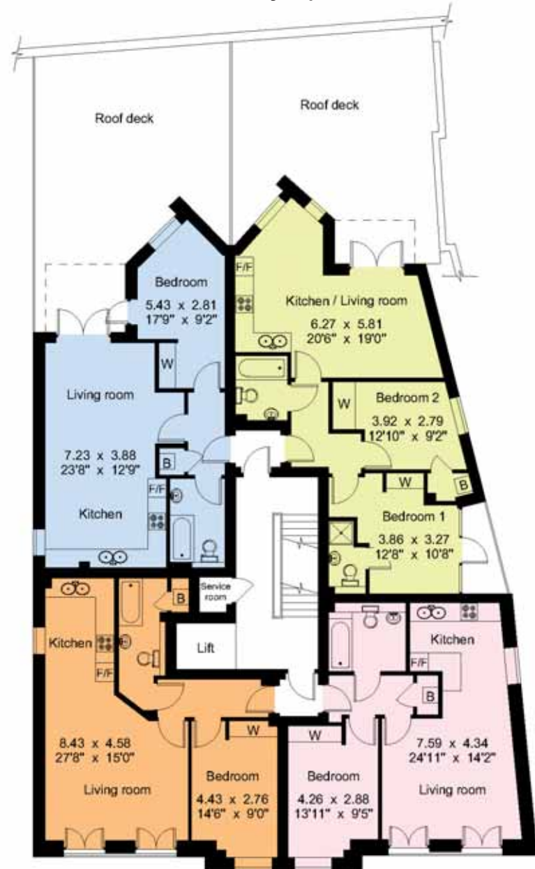
First floor - Foxbury Apartments
